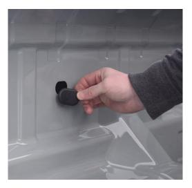
4. Insert upper clamp assembly into oval opening. Tighten bolts until bracket sits flush against bed of truck but can still slide freely.
