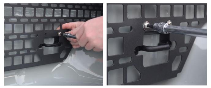
10. Check panel is aligned vertically and spacing around wheel well is consistent. When aligned, firmly tighten all bolts. Start with front and rear tie-down bolts, then tighten upper and lower brackets.
