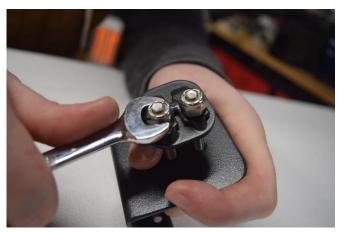
c. Back off both ¼-20 x 1-3/4 bolts until lock nuts are touching back of clamp plate.
