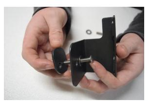
b. Thread lock nuts on back of clamp plate. Tighten nuts so one full bolt thread is exposed past the end of the nut.
