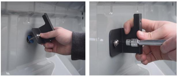
5. Attach lower bracket to middle tie-down location, using tie-down from step 1. Place tie-down ring in front of bracket and thread Torx bolts into truck. Tighten bolts but leave loose.
