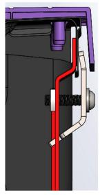
4. Insert GM cargo tie-down rings through oval opening in bracket, and into the oval opening in cargo box. When tie-down rings are inserted completely there will be an audible pop, indicating the forks have deployed. Loosely tie-down rings to remove excess play, and still allow movement.
