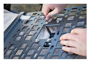
3. Take panel with installed brackets and lift it into place on the inside of the steel bed rail. The flange on the panel should sit flush to the inside of the top rail of cargo bed. Do not put panel between plastic bed cap and steel bed rail.
