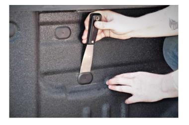
2. Install brackets to back of panel using two ¼-20 bolts and washers. Loosely tighten fasteners, so brackets can move freely.
