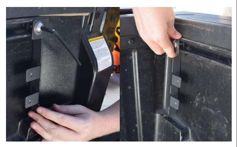
Place Panel in Truck. Panel should sit flush to brackets. Align holes in bottom of panel to holes in storage box frame. Once aligned, thread Torx bolts through panel and into storage box frame. Leave bolts loose.
