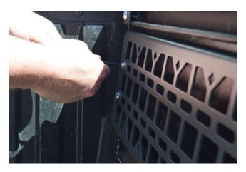
8. Align panel so storage box bolts are centered in slots and adjust brackets so they are vertical and completely engaged into cargo rail. Once aligned, firmly tighten all bolts.
