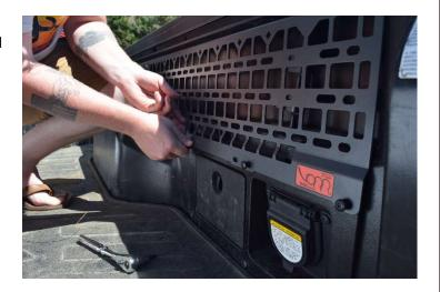
7. Bolt MAPS Panel to brackets front and rear using 1/4-20 screws and washers. Tighten bolts to remove play, but still allow easy adjustment.
