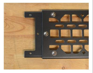
2. Join base panel and extension together using ¼-20 screws and washers. Align panels together so sides are flush and there is no gap between panels. Firmly tighten all six screws.
